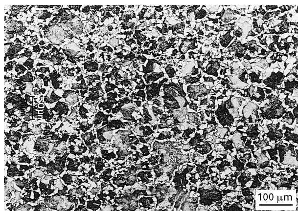
Figure 1 The fine-grained ferrite-pearlite microstructure of steel.
